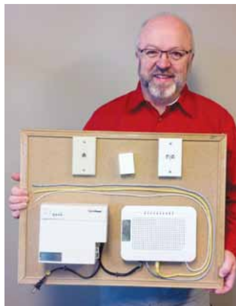
Duane Russell, Jefferson Telecom Plant Manager, holds a display of the equipment and wiring installed inside homes when they're converted to fiber.
